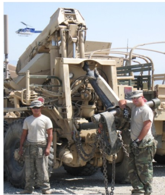
Above: PFC Dupa and SPC Wakly perform a PMCS on a M1984 Wrecker
